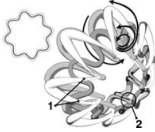
FIGURE 6. Schematic illustration of the main vortex line structure of vortex B during the nonlinear stage: depicted are inner, core, and outer vortex lines, giving rise to the secondary vortices (1: outer dipoles, 2: inner dipoles).
